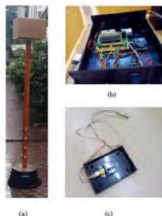
Figure 1. (a) Actual prototype of the flood monitoring system; (b) MCU circuit with Zigbee transmitter; (c) Zigbee receiver for the personal computer
